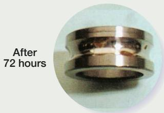
Corrosion-resistant coated bearings
