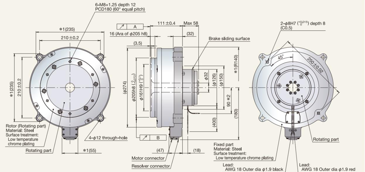
1. Dimensions marked with \*1 require an extra margin of 3 mm or more due to their casting surface.
