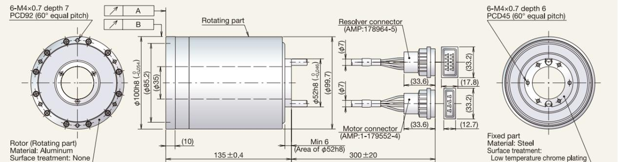
1. The bend radius of the motor cable lead (φ7) and the resolver cable lead (φ7) should be R30 mm or more.
