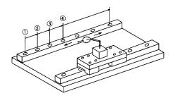
During installation, it is recommended that accuracy is checked to ensure smooth operation.
