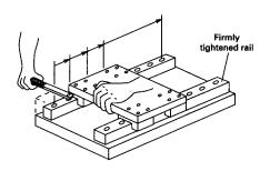
This method of assembly is for general industrial machinery where smooth linear motion is the overall objective. When precision accuracy is required, read on to the following procedure.
