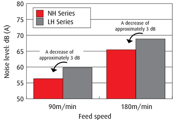
By re-examining the design for the ball circulation path, smoother ball circulation has been achieved, and noise level has also been reduced.
