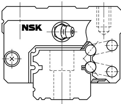
Note that rigidity defines resistance to external forces within a range of elastic deformation to deformation. In the context of linear motion devices, moment rigidity is the ability of a linear guide to support off-center loads. Moment rigidity depends on the guide series, size, preload and (as mentioned) ball groove arrangement geometry. Linear guide manufacturers list moment-rigidity values in catalogs.
