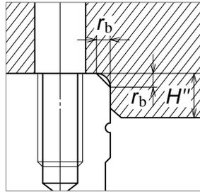
Fig. 11 Shoulder for the ball slide datum surface
