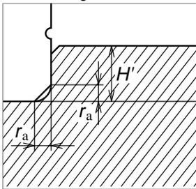
Fig. 10 Shoulder for the rail datum surface
